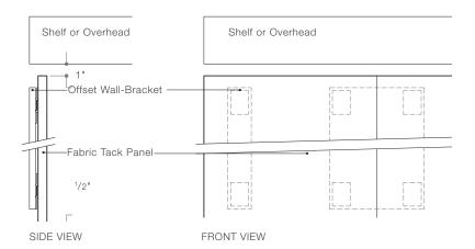
Tackable fabric panels are wall-mounted by means of offset wall-brackets.
